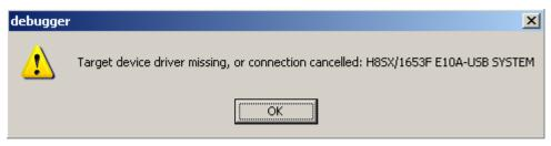
The drivers are E1USB.inf, hmseusb.inf, E1USB.sys, and hmseusb.sys. The .inf files should be in C:\windows\inf and the .sys file should be in C:\WINDOWS\system32\drivers. If not, try re-installing the E10A software. If the drivers are in the proper folders, check that the PC USB port is operating properly (with other devices) and try connecting the E10A directly to the PC if you are using a hub.
