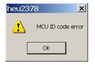
This error occurs when the wrong MCU is selected in the E10A connection window below.
