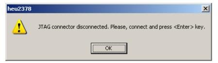
This error typically occurs if the JTAG connector from the E10A is not connected to the MCU. Ensure that the E10A is connected to the target device. You may have to reinitiate the connection sequence. If you are not using a Renesas RSK or EDK, then ensure that the E10A connector to the device is connected according to the instructions in the E10A "Supplementary instructions on using the E10A specific to the X family"; X being any MCU/MPU family.
