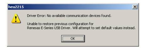
This error occurs when the E10A is not connected to the PC (or damaged), or it was previously disconnected in an unintended fashion. You can recover from this by connecting the E10A and target, wait a few seconds to be sure the devices has enumerated, and click <OK>. HEW will ask you for the driver, and then connection will proceed normally.
