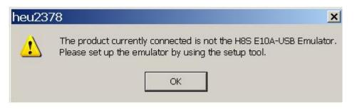
This error occurs when you do not have the proper version of firmware installed for the HEW E10A component. When switching the E10A between different families (H8S, H8SX, SH, SH2 etc), you need to update the firmware on the E10A to support that family by running the Emulator Setup tool.
